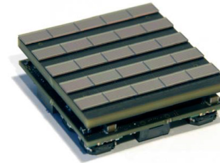
Front side: Tile of the first generation SPADnet sensor
